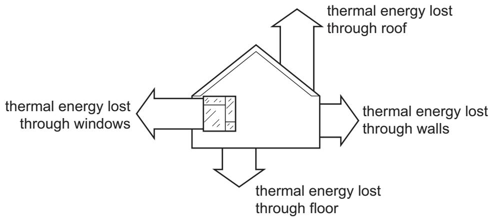
The heating system must supply more than 54 MJ of thermal energy to keep the temperature of the house constant.
