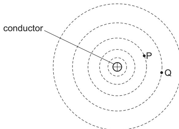
The current in the conductor is into the plane of the diagram.
